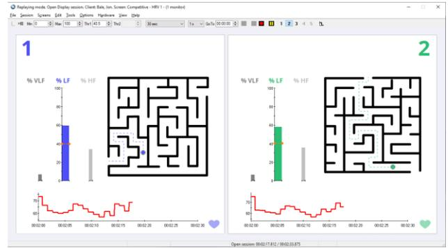
The HRV spectral frequency graphs are color coded for the three rhythms of activity: Very Low Frequency (VLF; dark grey), Low Frequency (LF; black or the player-specific color), and High Frequency (HF; light grey). The Low Frequency graph also contains a feedback threshold that controls the player's feedback animation. This threshold is manually set.
