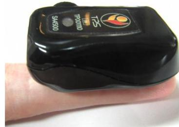
4. Secure the TPS sensor to your finger by wrapping the fabric strap around your finger and back over the TPS sensor. The fabric strap is perforated with loops. Slip an appropriately positioned loop onto the central hook of the sensor.
