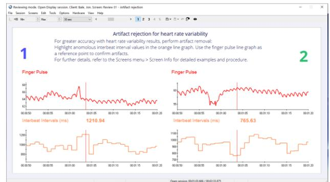
Artifacts are patterns in the signal that are not created by the physiological process of interest. They happen when the signal gets distorted by movement or other sources of noise. Artifacts can cause errors in the signal processing calculations and make the data analysis unreliable. Prior to generating a report, it is always a good idea to review the recorded HRV data and correct it for artifacts. Doing this normalizes the data and ensures that the program generates correct statistics.
