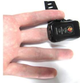
3. The sensor should be placed at the end of your finger. The two metal plates on the underside of the sensor rest against your skin as shown.
