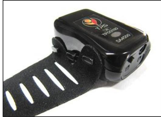
2. Place the TPS sensor on your finger so that the sensor label faces up and the ON button points toward your hand.
