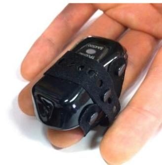
We advise to apply the sensor at least 2-3 minutes before recording a session. This is due to the temperature sensing component, which requires that time to “warm up” to the client’s current temperature.
