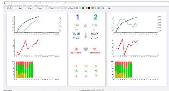
The HRV spectral frequency graphs are color coded for the three rhythms of activity: Very Low Frequency (VLF; yellow), Low Frequency (LF; green), and High Frequency (HF; pink).
